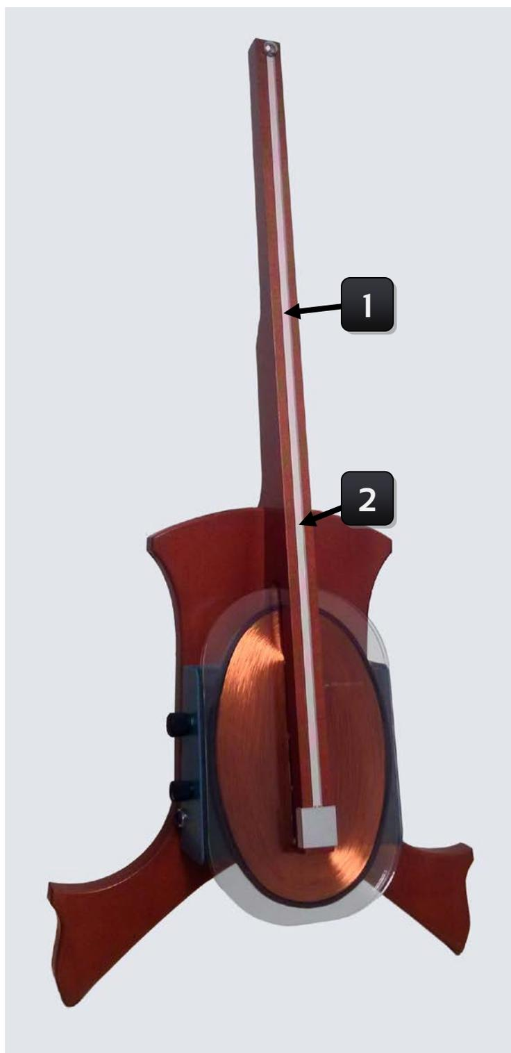
Notes are chosen by pressing along the resistive ribbon “string”. Like an acoustic string, higher notes are located further down the string, and notes become more compact going down the string. *Glissando* and *Vibrato* can be achieved by sliding or vibrating on the ribbon while bowing.
