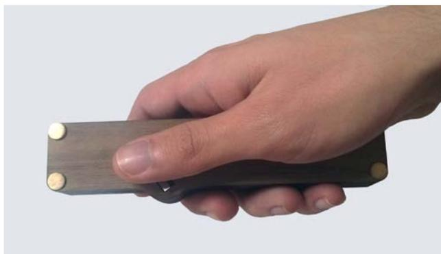
The magnetic bow is held as shown above. The right hand wraps around the body of the bow, and the thumb is placed over the switch, such that rocking the thumb left and right presses the switch.
