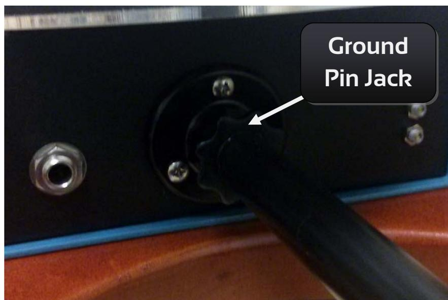
The instrument is held up during play using the included **Ground Peg**. To extend the ground peg, twist the middle grip, pull to desired length and twist again to tighten, just like a microphone stand. The peg is then threaded into the **Ground Pin Jack** located on the underside of the Magnetic Cello.
