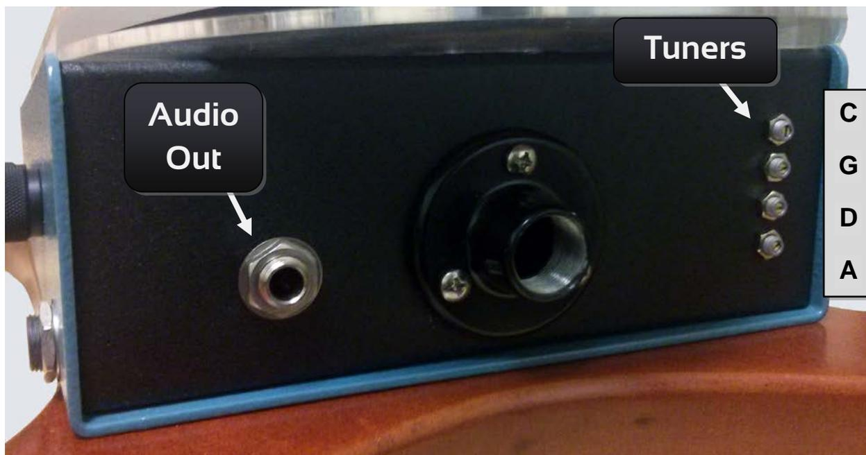
Also on the underside of the instrument are the **Audio Out** and the **Pitch Tuners**. The audio out jack accepts standard  $\frac{1}{4}$ " audio cable plugs (not included). We recommend connecting the output of the Magnetic Cello to a bass or piano amplifier rather than a guitar amp, to take full advantage of the instrument's low range.
